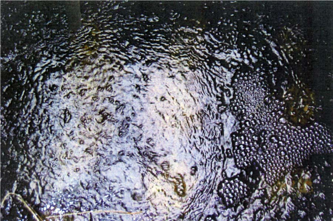
Incoming sewage, dark color, includes fats/oils/grease (FOG)
